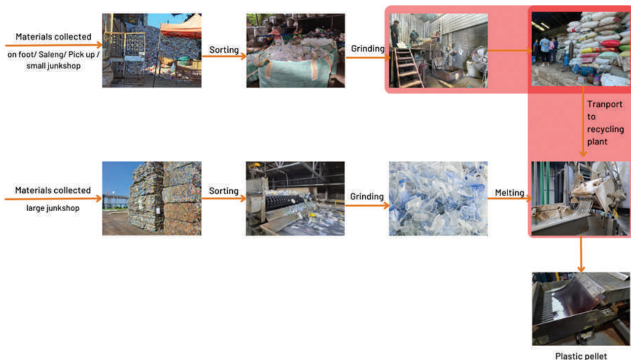
Figure 14. The plastic pellets production process and the hotspot area for the leakage of plastic pellet / scraps
