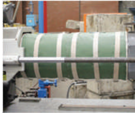
(b) Insulation layer is installed on extruder
