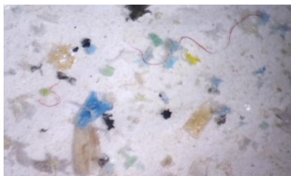
Figure 9.3. Different Shapes of Microplastics Extracted from the Influent of a Wastewater Treatment Plan in the Philippines
