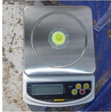
Digital scale (The yellow round tool is a horizontal leveler, which helps to measure weights accurately.)
