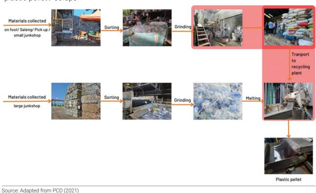
Figure 14. The plastic pellets production process and the hotspot area for the leakage of plastic pellet / scraps
